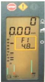
The corner post display will display information such as speed, engine RPM, selected gear and the status of the main components, such as the PTO, differential lock and front traction, among others.
