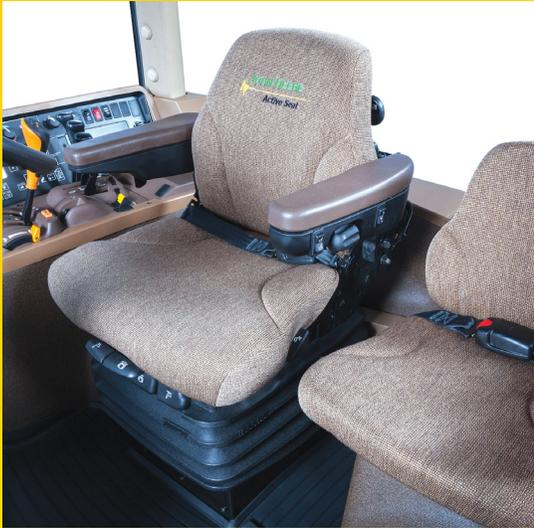
Combined with air suspension and electro-hydraulic technology, ActiveSeat™ reduces vertical seat movements by up to 90%, providing better ergonomics and comfort to the operator, improving quality and safety during operations.
