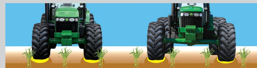
Tractor with conventional MFWD axle 7J Series Tractor in sugarcane applications with a 3 m axle
