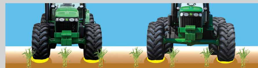
Tractor with conventional MFWD axle 7J Series Tractor in sugarcane applications with a 3 m axle
