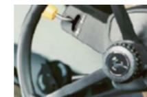
*The reverser, on the left side of the steering wheel, allows the forward/reverse direction to be switched without using the clutch, enabling agile maneuvering.*
